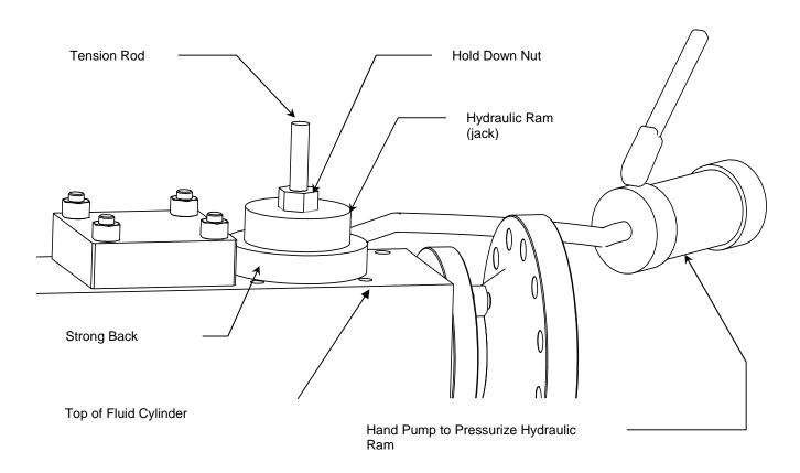
Figure 10: Hydraulic Power used to Remove Valve Seat
