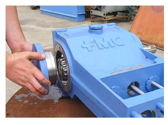
(19) that will remain attached to one housing. It may be necessary to tap on the housing with a rubber mallet to free it from the power frame after the hex head cap screws have been removed.
