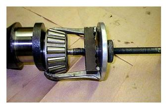
replaced, the corresponding cup or cone should be replaced as they are a matched set.
