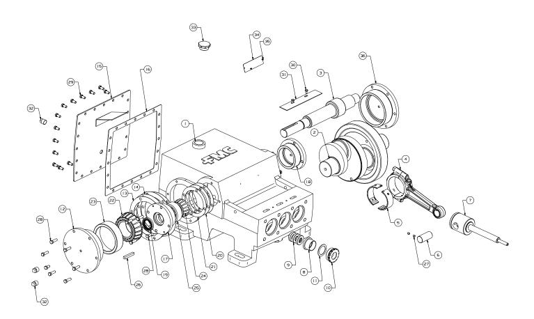
Figure 3: Power End Components
