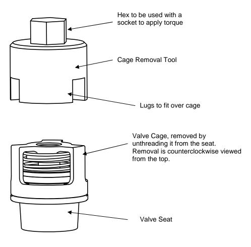
Figure 7: Valve Disassembly
