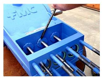
3. For L09 through L16 models, pull the seal holder (8) out of the pump frame and slide off of the rod. It may be necessary to insert a screwdriver or pointed tool into one of the holes in the seal holder on the L09 to help extract it from the power frame. For L11 through L16, it will require using two screwdrivers to slide the seal holder out of the recess. A slight rocking motion on the seal holder may aid in removal.
