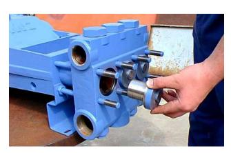
5. Some pumps may be equipped with a single cover plate that secures all three cylinder covers. For these models, all eight nuts (61) must be removed to facilitate removal of the cylinder covers (54). For some L06 models with no cylinder covers, the fluid cylinder (37) must be removed to access the pistons.
