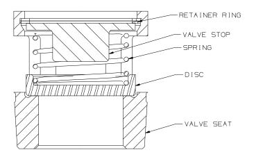
Figure 13: Typical L Series Disc Valve Assembly
