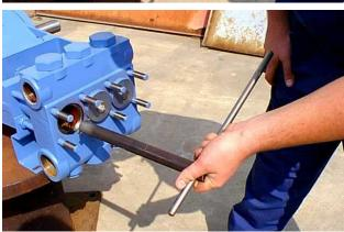
8. Pull the piston assembly free of the pump using a combination pulling and twisting motion.
