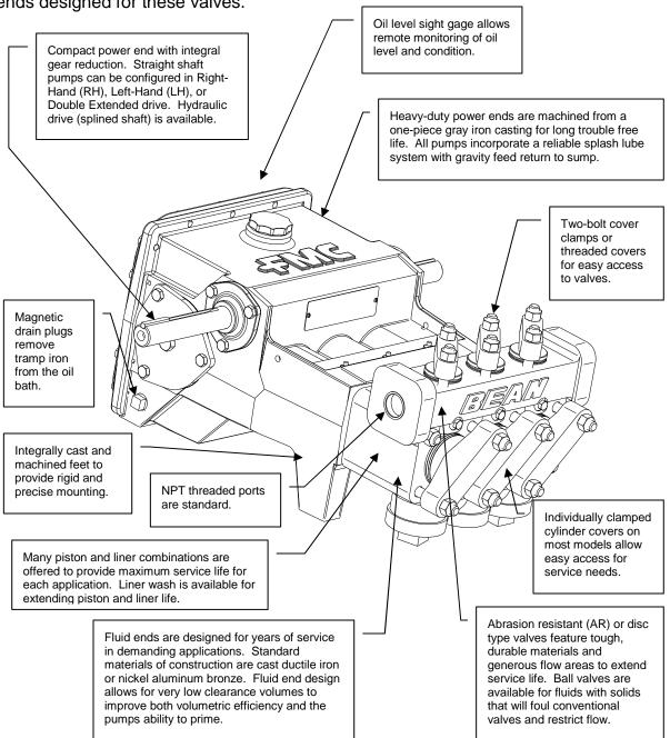
Figure 1: L11 – L16 Pump Assembly with Pinion Shaft
