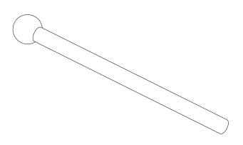
Figure 14: Illustration of the P534694 and P534695 Ball Knock Out Tools
