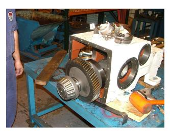
frame and remove. The crankshaft should be handled carefully to prevent the critical bearing surfaces from being scratched or damaged.
