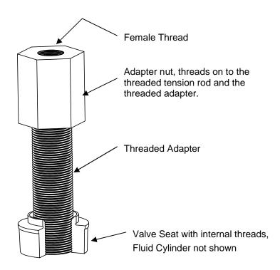
Figure 12: Threaded Tool in use
