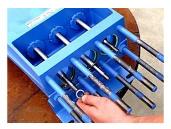
12. Tighten all fasteners to the values specified in Fastener Torque Requirements, Section 11.0 of this manual.
