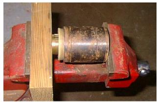
Service Tip – Press the piston assembly into the liner until the sealing lip has just entered the front of the liner. Use a small amount of glycerin on the ID of the liner to help lubricate the piston during installation. After the liner has been installed in the pump power frame, drive the piston assembly fully to its stop using the FMC piston tool (A5049) and a rubber mallet.
