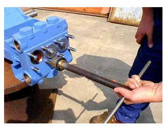
9. Place the flats on the bottom of the piston holder (41) in a vice or clamp securely. Using the FMC piston tool, unscrew the piston retainer nut (43) and remove. The piston cup (40) and piston retainer (44) may now be removed.
