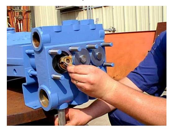
Picture 2: Removing the valve from the fluid cylinder
