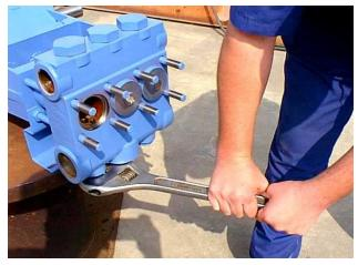
4. Remove the three valve covers (49), the threaded version is shown, or remove the six valve cover nuts (53) holding the valve cover clamps (51) and then remove the three valve covers (49) from the fluid cylinder. NOTE: Pumps that have threaded valve covers do not require removal of nuts and clamps.
