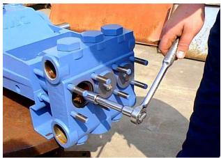
7. Following the hex piston nut (42) removal, use the FMC piston tool (A5049) to pull the piston assembly from the cylinder (39). Insert the FMC piston tool inside the cylinder until flush with the face of the slotted piston retainer nut (43). Twist the tool to engage and lock the tabs of the tool inside the mating slots in the retainer nut.
