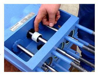
4. Remove the seal retainer gasket (11) from the power frame. Inspect the seals (9) and note the orientation of the seals prior to removal. The seals may now be removed from the seal holder and discarded.
