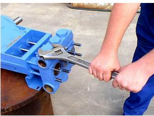
5. The cylinder covers (54) on most "L" series pumps allow access for inlet valve removal. For these pumps, remove the cylinder covers as described in section 10.1, steps 1 through 4. Some pumps may be equipped with a single cover plate. Refer to 10.1, step 5.
