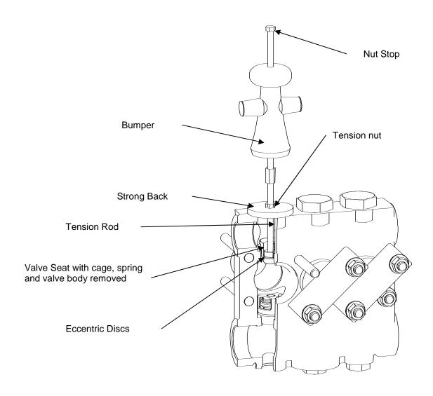
Figure 9: Removing the seat
