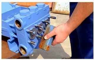
4. To access the piston cup seals (40), the cylinder cover clamps (57) must be removed (except as noted for L0918 in service tips above and some L06 models). Remove six of the nuts (61) holding the cylinder cover clamps (57) in place, and then remove the cylinder covers (54). Do not remove the two nuts (61) on the opposite corners of the fluid cylinder, as they keep the cylinders (39) and fluid cylinder mounted on the pump during this operation.
