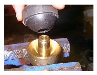
11. Reverse steps 3 through 10 to rebuild the pump after worn or damaged components have been replaced. FMC recommends that all seals and gaskets that are disturbed during the service procedures be replaced. This includes the rod seal o-ring (45) that is located on the piston/crosshead rod (shown) directly behind the piston assembly. Some pump models have the o-ring in a groove in the piston holder instead of a separate seal holder. Lubricate the piston cups and piston rods during assembly.
